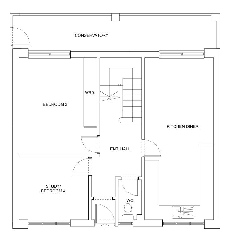
**GROUND FLOOR INTERNAL LAYOUT** (AS PROPOSED) scale 1:50
